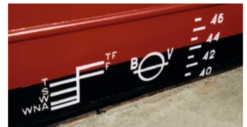
The Plimsoll line identifies the Classification Society
