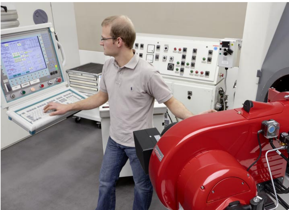
All marine burners are fully tested on special test rigs prior to delivery
